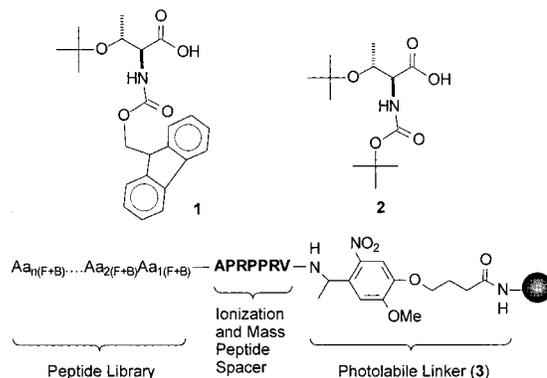
**Figure 1.** The construct of peptide and peptide libraries containing an IMP spacer and the photolabile linker **3**. A 9:1 mixture of orthogonally protected amino acids (e.g., Fmoc (**1**) and Boc (**2**)) were used in the ladder synthesis of the glycopeptide libraries.
