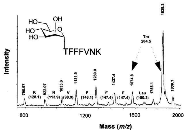
**Figure 6.** The MALDI-TOF-MS spectrum of the monoglycosylated active peptide **23** showing the peptide ladder sequence and carboxylic acid label, lauric acid (Lau), which indicates that the glycosylated residue is Thr( $\alpha$ -D-Man) (Tm) and is at the N terminus. The peak at 1936.1 represents the peptide-TFA adduct.
